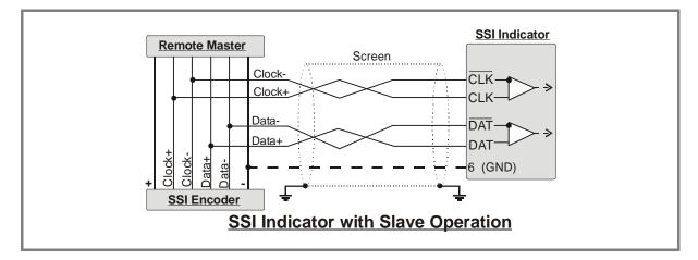
Set registers "Bits", "Format" and "Baud" according to the encoder you use.
